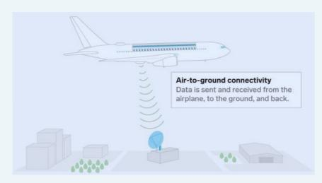
**Ground-based connectivity also** Air known as to Ground connectivity works exactly like our conventional mobile network. It has a base station on the ground with antenna arrays upwards to facing maintain signal connectivity to moving airplanes.
